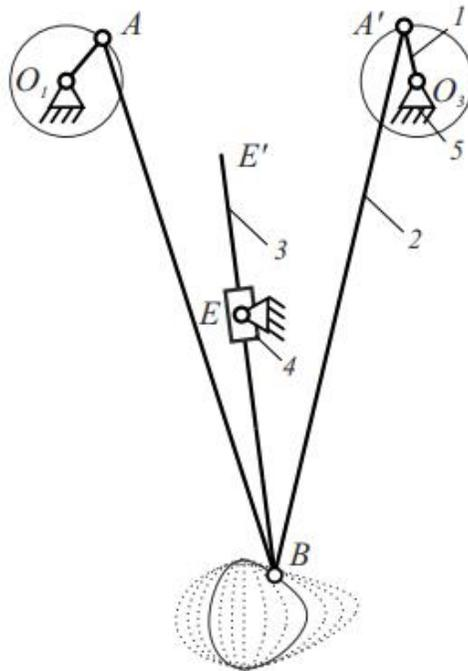
The femur mechanism of the cheetah robot leg
